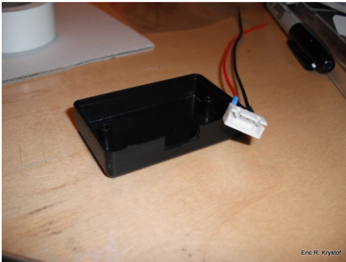
LED Enclosure Box with LiPo balance port connector
