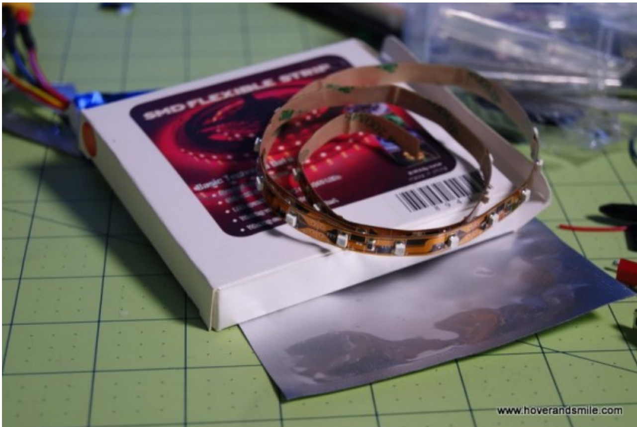
A SMD LED Strip - Hook up 12 volts and Go!
